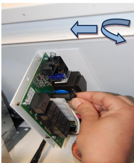
**PCB replacement:** Open the service panel and simply unscrew the power plate from the inside of the air curtain to remove it and make the necessary repairs.
