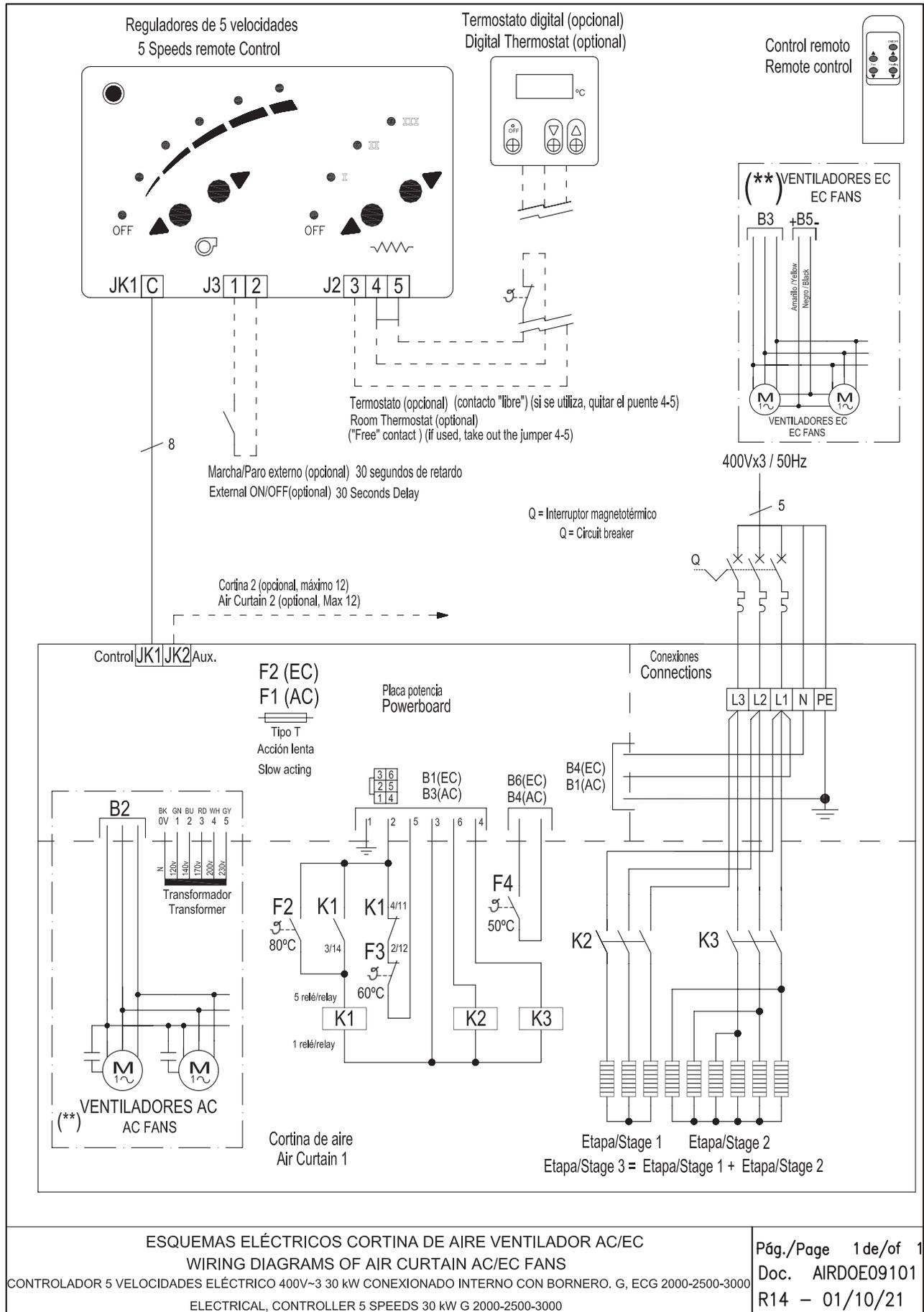
In case there is a need to connect the curtain to a PLC, the corresponding diagram is attached
