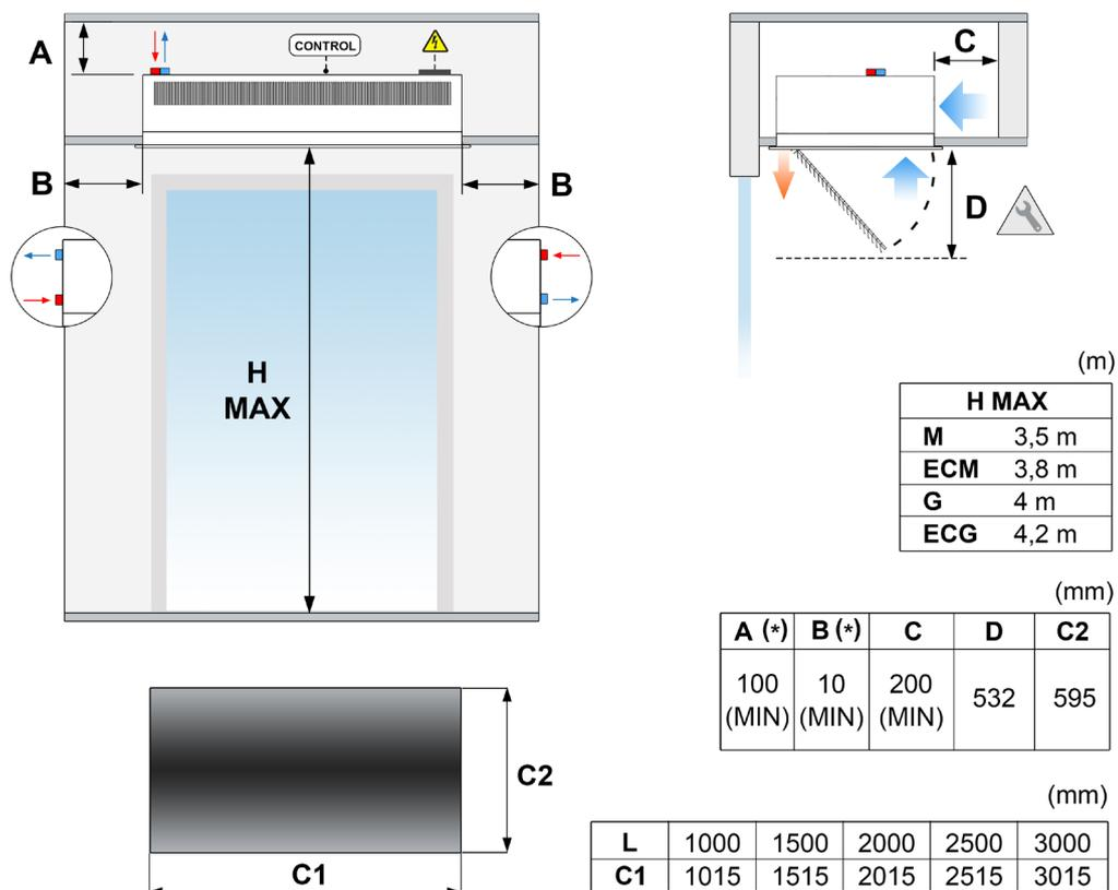
H MAX. Maximum recommended range, MIN. Recommended minimum distance
