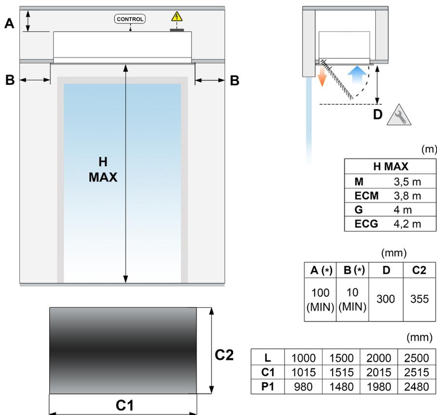
H MAX. Maximum recommended range, MIN. Recommended minimum distance
