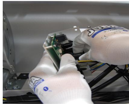
**Power board replacement:** open the service door and unscrew the power board from the inside of the air curtain to remove the plate and carry out the necessary repair.
