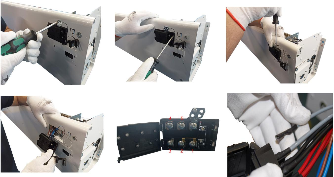
To remove the battery, remove the suction grille (process shown in water battery). Remove the screw from the connecting phase to gain access to the battery. Unscrew the fixing screws (see table at the bottom of the page to count the screws to be removed), disconnect the PRBEO cables from both parts of the battery and remove the battery with both hands.
