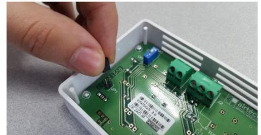
**Delay thermostat:** when the device is stopped with the heating on, there is an increase in temperature inside it that could damage its components due to the thermal inertia of the electrical resistors. To avoid this, the curtain continues to work up to 90 seconds after stopping; and if when stopping the curtain, the temperature rises above 50 °C, the equipment goes to maximum speed and does not stop until the excess thermal energy is evacuated.
