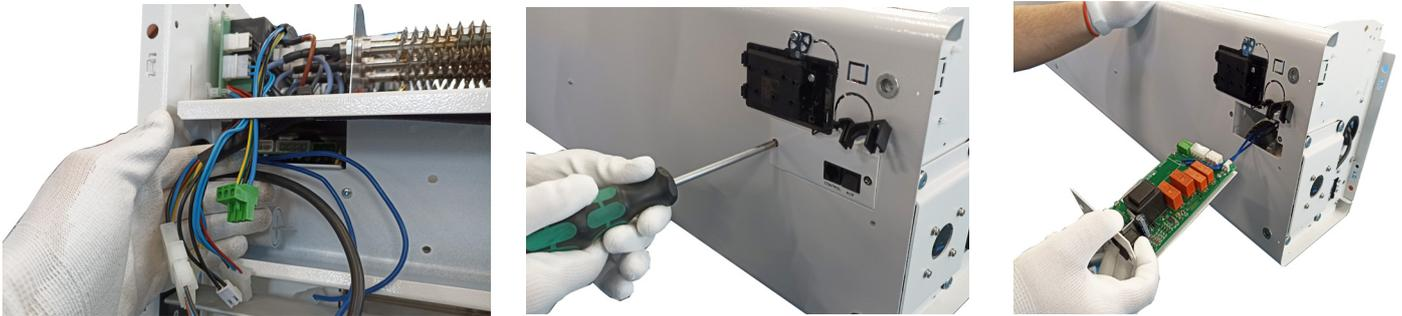
**Change fuse:** remove the pcb from the curtain for better maneuverability, remove the fuse protection casing and remove the fuse by hand or with the help of a screwdriver. Proceed to make the replacement and follow the reverse process to leave the curtain functional.
