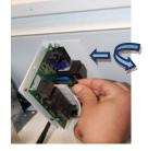
**PCB replacement:** Open the service panel and simply unscrew the power plate from the inside of the air curtain to remove it and make the necessary repairs.
