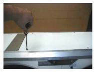
2.- Remove the panel carefully. If available, use a sucker, if not a screwdriver will do.
