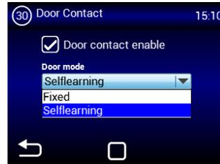
**Selflearning**- available only in automation and active function mode (Auto speed control), depending on the number of open doors it optimises the period in which the shutter is in operation, even when doors are closed.
