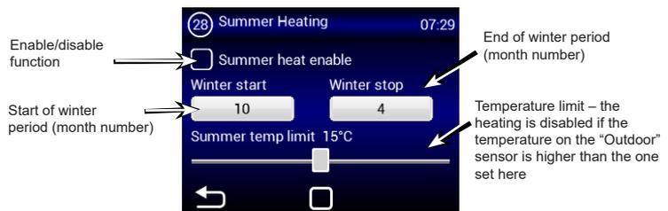
If the outside temperature sensor is not set, the "summer heating" mode will operate only according to the selected time and the temperature will not be taken into account
