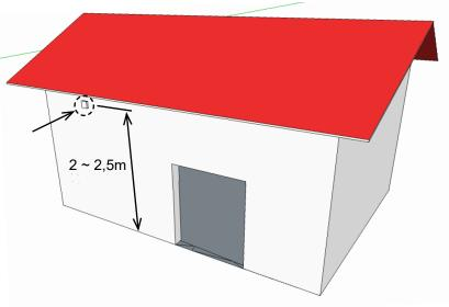
It is recommended to install the outdoor temperature sensor on the north side of the building, protected from direct sunlight or other unwanted heat radiation.
