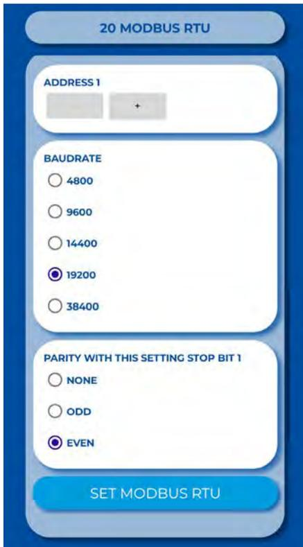
The MODBUS menu is used to set the Modbus communication.
