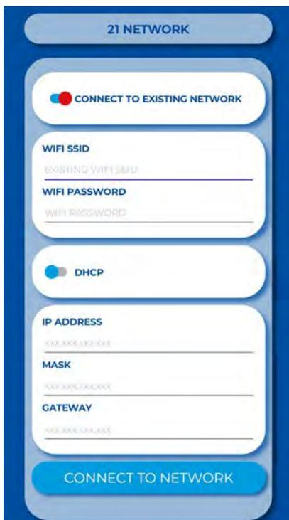
The NETWORK menu is used to set up the control's network communication so that you can connect to multiple devices from one local WiFi network.
