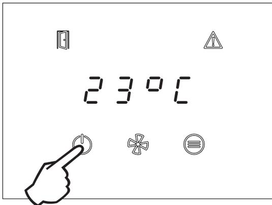
The unit starts by pressing the power-on symbol for 2 seconds.
