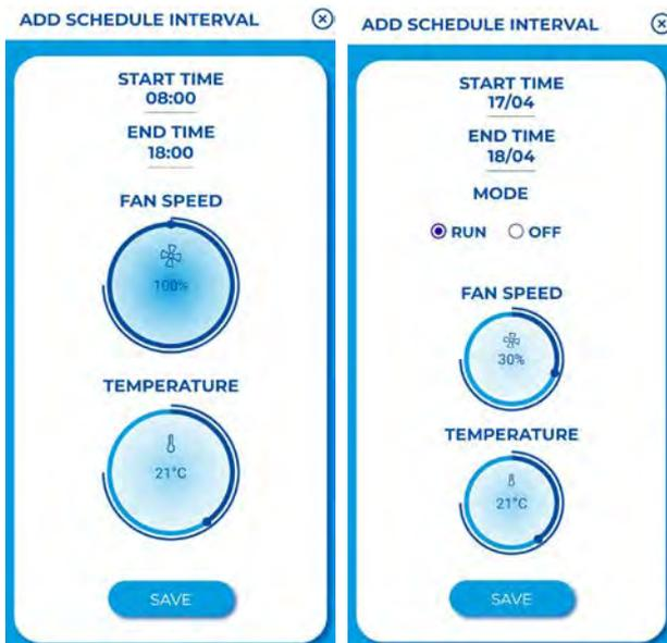
⊗ Touch to set individual intervals of ventilation (time ON/OFF, vent. mode, vent. level, temperature)
